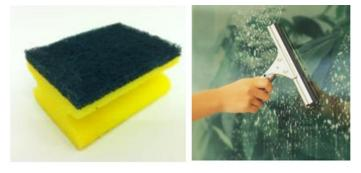
As shown in figure above, the blue face of a sponge can only be used to clean the aluminum frame of the modules. It cannot use to clean the glass side as it will scratch up the glass which resulted in reducing the output power.
